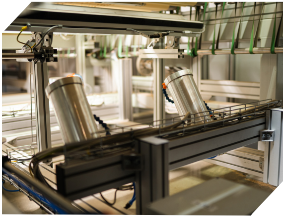
Cameras monitor both faces and all edges of the board
