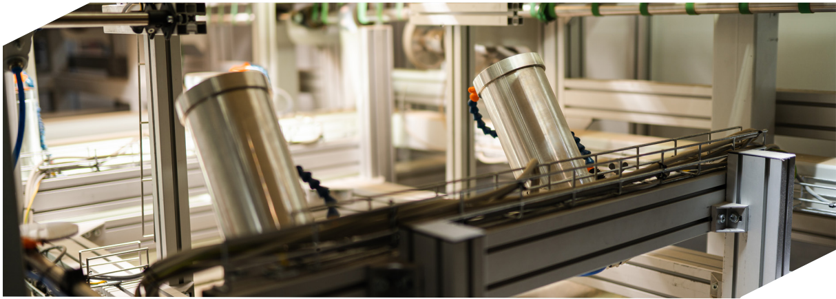
Cameras monitor both faces and all edges of the board
